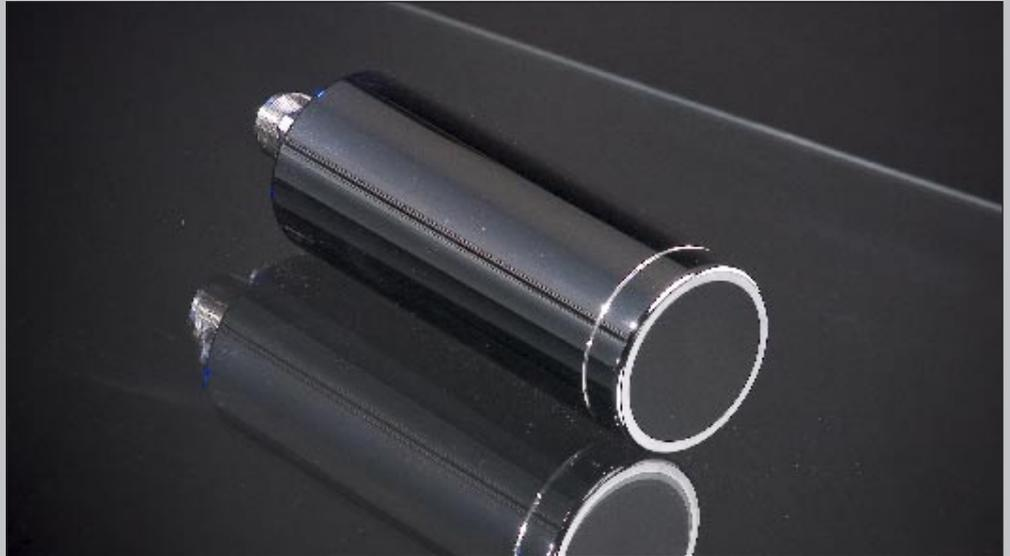
The Oceanscan Multi-Return Altimeter fulfills many of the sonar data capture requirements of the oceanographic and scientific communities. This unit differs from most Altimeters of the "first-return" type by digitising the receiver output at high speed into a FIFO memory. The range to the sea-bed is then calculated in the digital domain by the mathematical processing algorithm programmed into the internal RISC microcontroller.
